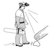
7 Take great care when cutting a tree that is in tension. A tree that is in tension may spring back to its normal position before or after being cut. If you position yourself incorrectly or make the cut in the wrong place the tree may hit you or the machine and cause you to lose control. Both situations can cause serious personal injury.
